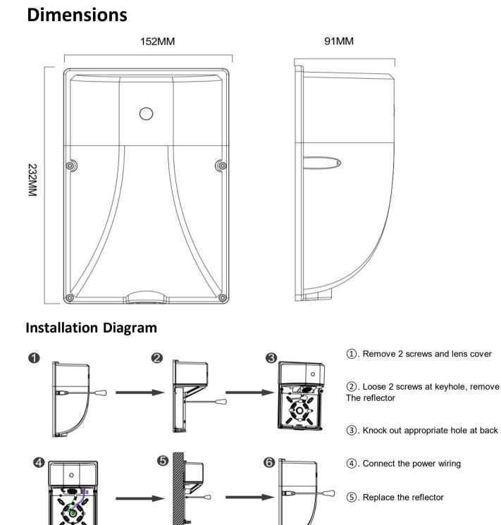
6. Fix the lens cover by screws
