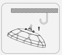
2. Put the ring into the mounting hook
